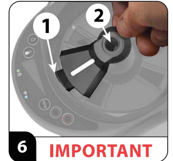
1. Place the front edge of **locking cover** in the recess in the inside/front of the powder container, **UNDER THE TAB**.
