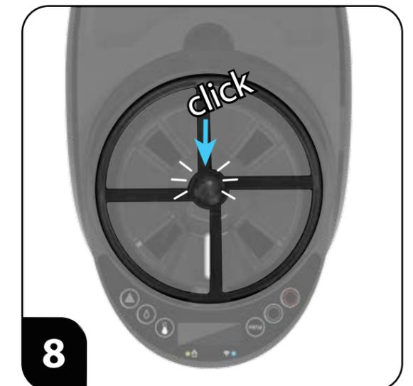
Now place the **stirring wheel** on the axle and push down firmly until you hear a **click**. Make sure the stirring wheel is snapped in place and does not lift up easily.
